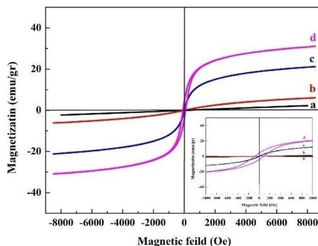
**Figure 4.** Magnetization curves as a function of magnetic field for NiFe<sub>2</sub>O<sub>4</sub> nanoparticles (a) as prepared and annealed at (b) 500°C, (c) 700°C, and (d) 900°C.
