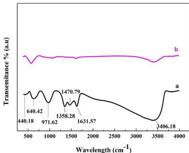
**Figure 3.** FTIR spectra of a) as-prepared b) annealed at 900°C NiFe<sub>2</sub>O<sub>4</sub> nanoparticles.
