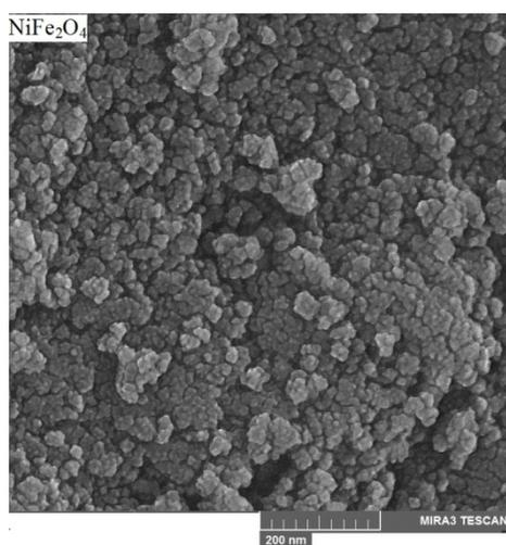
**Figure 2.** FESEM image of NiFe<sub>2</sub>O<sub>4</sub> nanoparticles, which annealed at 900°C.
