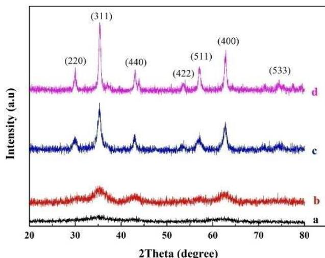
**Figure 1.** X-ray diffraction patterns for NiFe<sub>2</sub>O<sub>4</sub> nanoparticles (a) as-prepared and annealed at (b) 500°C, (c) 700°C and (d) 900°C.
