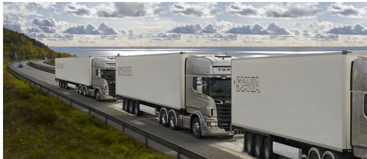
Figure 1: Three heavy-duty vehicles platooning to collectively reduce fuel consumption.
