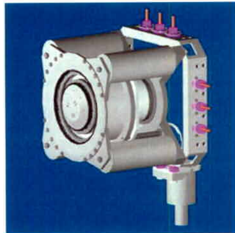
Figure 2. A CAD drawing of the VHITAL 160 with feed system.
