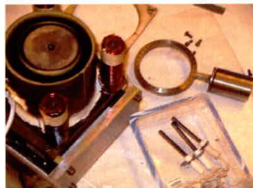
Laboratory SPT thruster with modified anode, bismuth vaporizer, and electrical heaters.
