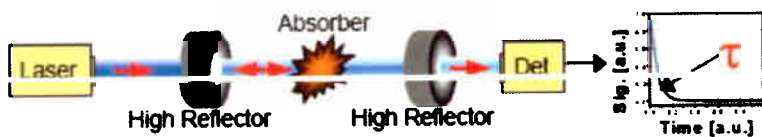
Figure 28. Schematic diagram of cavity ring-down spectroscopy (CRDS).
