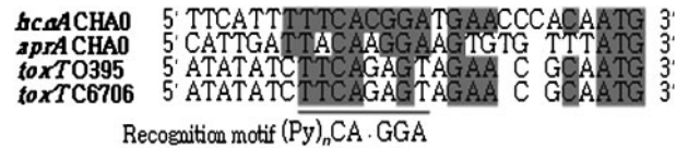
Fig. 4. Alignment of the regions containing the ribosome-binding site of hcnA and aprA genes of P. fluorescens CHA0, and toxT genes of V. cholerae O395 and C6706. In each case, translation is initiated at the ATG codon shown at the 3' end.
