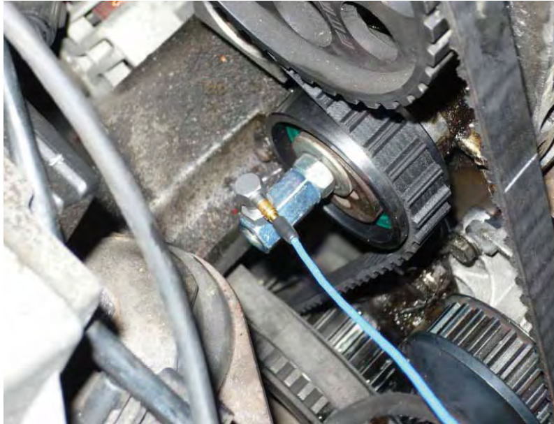
Fig. 1. The view of the timing gear's drive after dismantling the shield and the place of fastening of the vibrations speed detector
