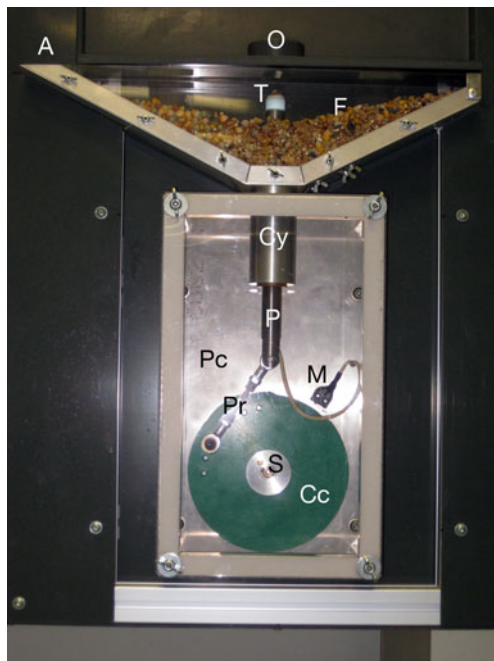
Fig. 4 Grain lifter, realized as a crankshaft (consisting of a crank cheek, piston rod, and piston). The piston is shown in its waiting position, beyond the reach of the subject. A, aperture for refilling food; O, elevated feeder outlet at the bottom of the Skinner box; T, top of the piston, with feeder light and accumulated food; F, food reservoir; Cy, guide cylinder; P, piston; Pc, Plexiglas case; M, microswitch; Pr, piston rod; S, sliding clutch; Cc, crank cheek
