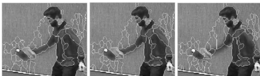
Figure 31. Watershed line computed on the precedent filtered relief (from left to right: r_0 = 5, 10, 20 ).
