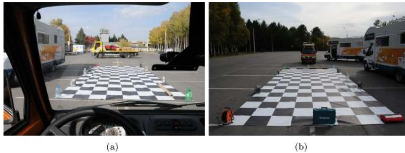
Figure 5 Stereo cameras calibration procedure with the chessboard pattern in a car park in Barnaul (Russian Federation): (a) internal view and (b) external view (see online version for colours)
