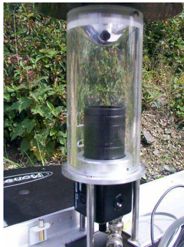
Figure 2: The omni-directional camera: the “normal” camera (bottom) and the hyperbolic mirror (top) linked by a perspex tube
