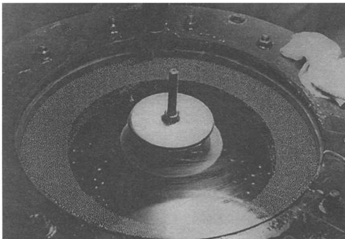
Figure 2. Condensed stable state of a mixture of liquid-solid particle in a vortex chamber. Note the dense, homogeneous particle layer near the periphery, forming a rotating axisymmetric fluidized bed.
