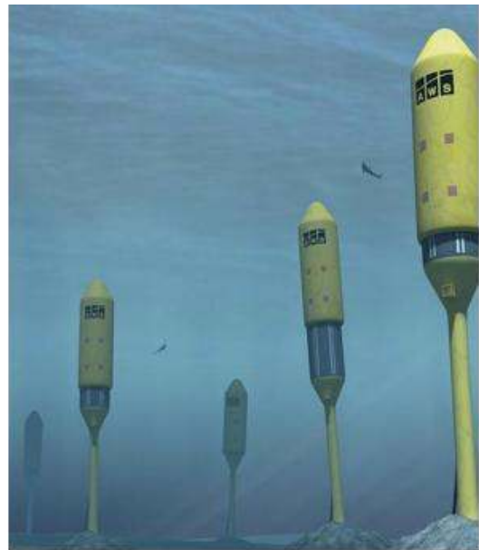
Figure 8. Artist's rendition of an array of Archimedes Wave Swing point absorbing WECs [14].
