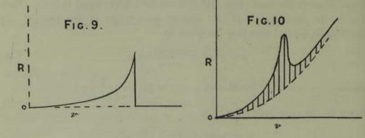
We can obtain a better estimate of equation (27) by taking an experimental curve for a model in deep water, and then building up curves for different depths. We must first put (27) into a form suitable for comparison with deep water results.
