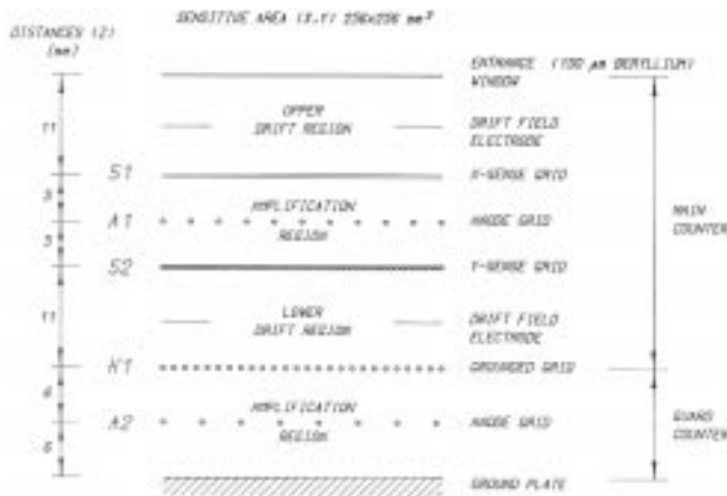
Fig. 4. Schematic diagram of the WFC detector showing the configuration of the main and the guard counter. The guard counter serves to reject background and spurious events
