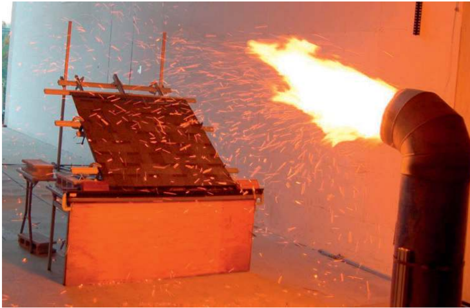
Fig. 2. Snapshot of NIST (National Institute of Standards and Technology) firebrand generator operating in the BRI (Building Research Institute) wind tunnel ( 9 \text{ m s}^{-1} wind). The target for the firebrand assault is a section of a roof.
