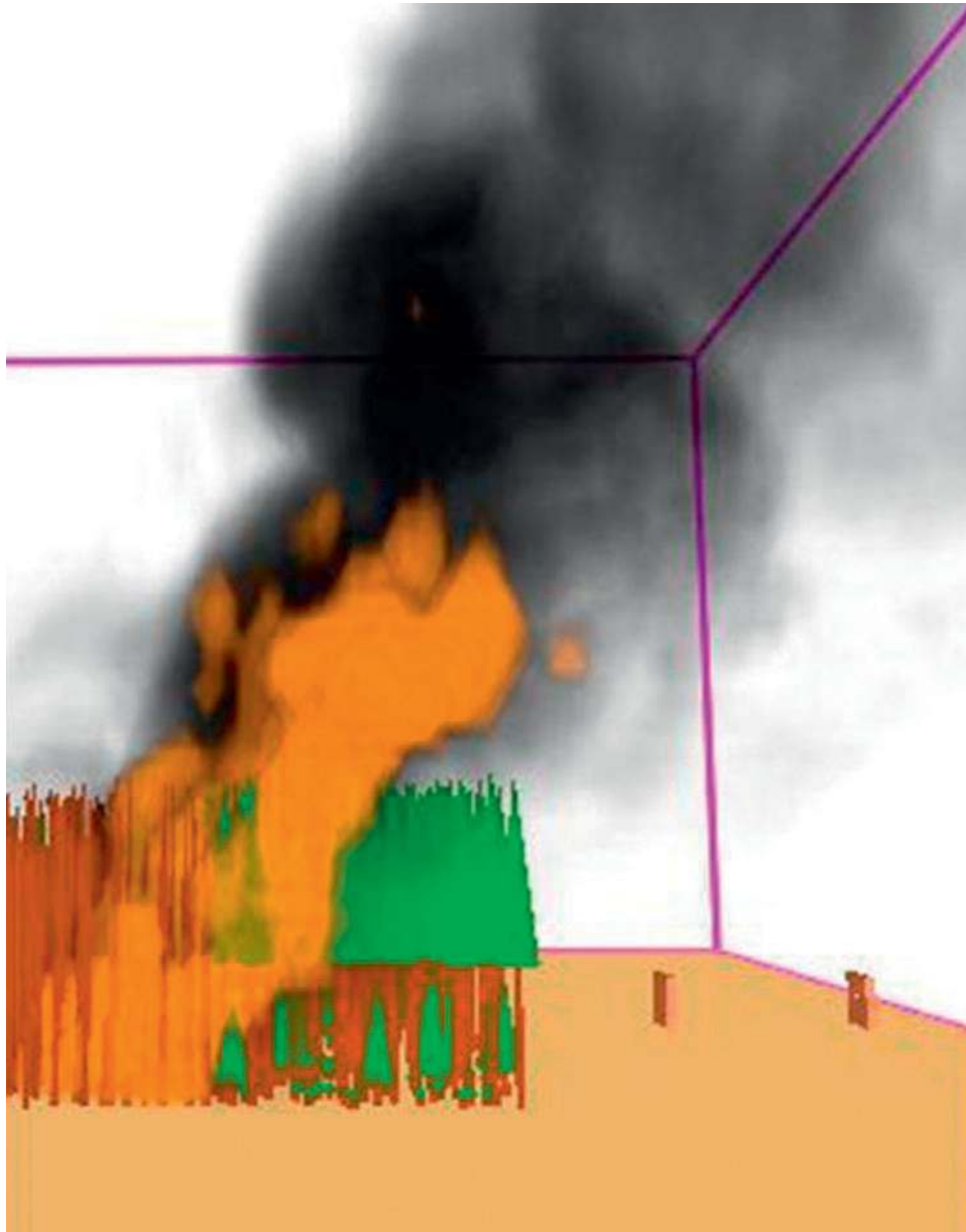
Fig. 4. A snapshot from a Wildland–urban interface Fire Dynamics Simulator (WFDS) simulation of a crown fire based on the experiments reported by Cohen (2004). Mock walls can be seen at 10 and 20-m distance from the edge of the wildland plot.
