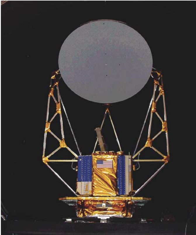
Fig. 1. WindSat payload in the thermal/vacuum chamber. The cold sky reflector has been removed in this picture.
