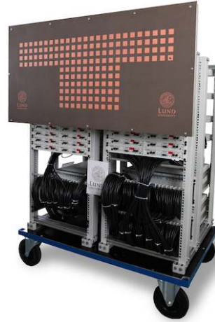
Fig. 7. Left: Side view of the mechanical assembly of the BS. The two racks sit side by side (not as shown) with the SDRs facing the same direction (towards the antenna array). Two columns of USRP SDRs are mounted in each rack, totaling 50 of them. Right: The assembled LuMaMi testbed at Lund University, Sweden.
