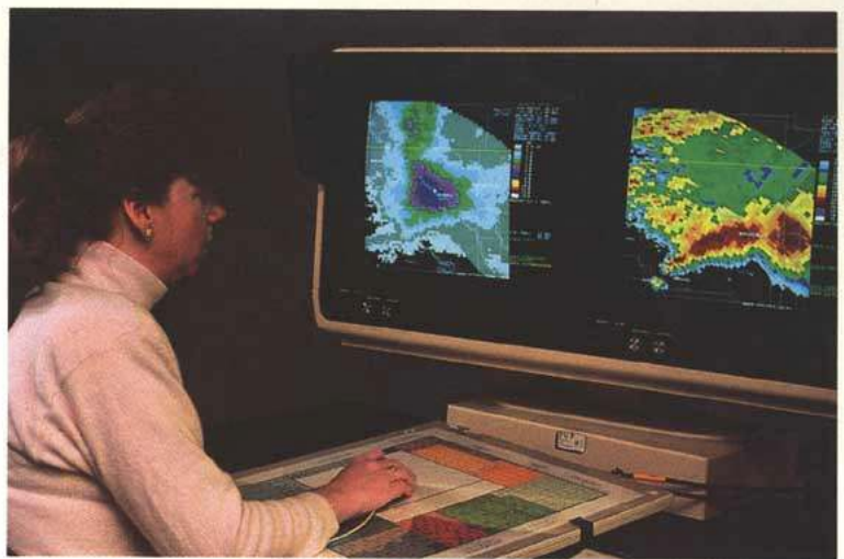
FIG. 6. A WSR-88D PUP workstation. The forecaster/operator displays products on the twin 19-inch color monitors. The graphics tablet and puck are used to interact with the displays.
