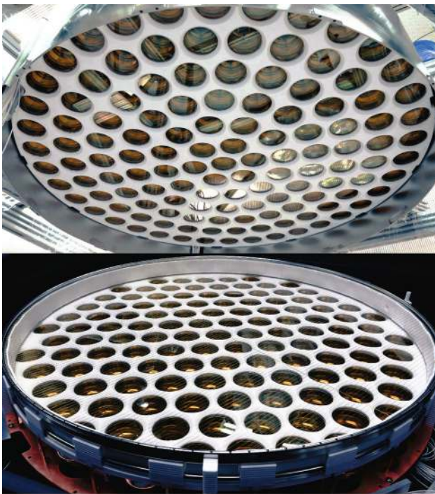
Fig. 4 The top and bottom PMT arrays are equipped with 127 and 121 Hamamatsu R11410-21 tubes, respectively. The top array is installed inside a diving bell, used to maintain and precisely control the LXe level. The bottom image also shows the cathode and the bottom screening electrode, installed in front of the PMTs
