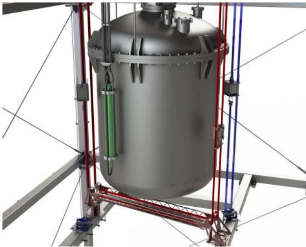
Fig. 12 The deployment system for external calibration sources. Two belts (“I-belts”, blue) allow for vertical movement of sources inside their W-collimators, while one belt (“U-belt”, red) reaches areas around the detector bottom. The DD-fusion neutron generator (green) can be vertically displaced along the cryostat
