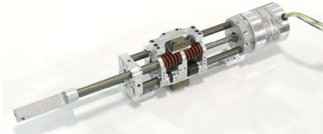
Figure 2: Linear Series Elastic Actuator. All 12 actuators in the robot are identical except for the plunger ends.
