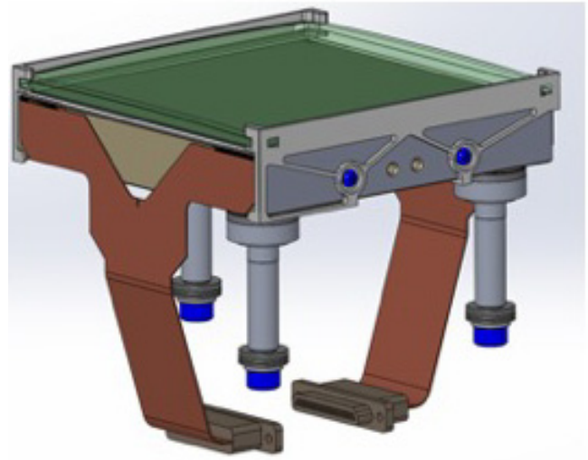
Figure 12. A science CCD with its field flattener held between titanium frames, showing signal cables and triad of posts that secure the package against cold plate defining points.
