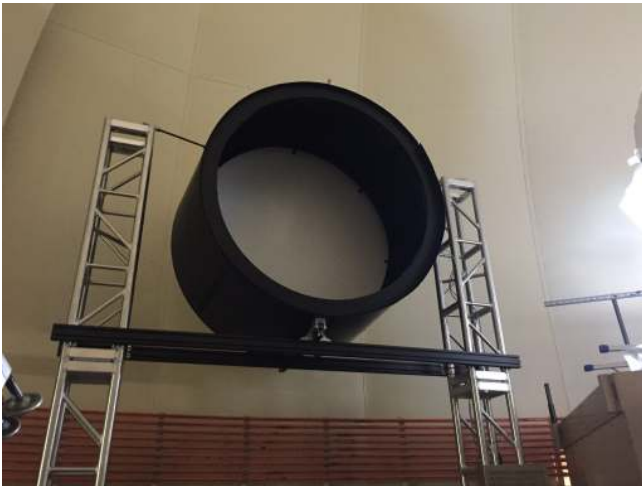
Figure 21. The ZTF flat field illuminator installed in the telescope dome.
