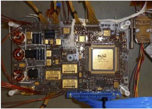
Fig. 4.30: FM BepiColombo DPU SCU Board/Eurocard of 100 \times 160 \text{ mm}^2 . SCU is a high-rel DPU FPGA processor card such as the ones matured on the BepiColombo Mission / SERENA DPU in which the DPU had to control and support a similar S/C data handling bus and four sensors units.
