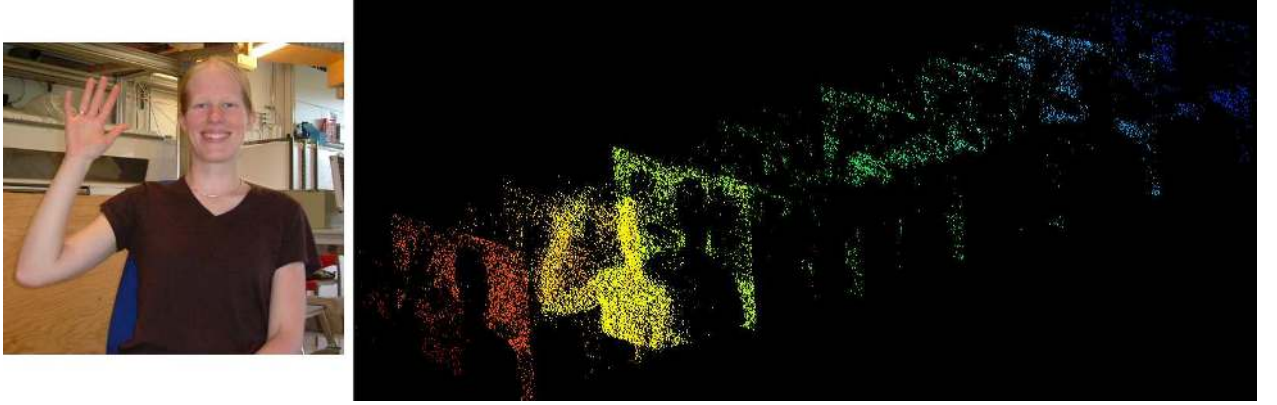
Figure 3 Indoor scene as observed by a conventional digital camera and by a 3D camera system at 5ms exposure time. The output is displayed by the software CamVisPro. The spurious “walls” at discrete depths are artifacts produced by pixels with low amplitude, see section 4.3.2.
