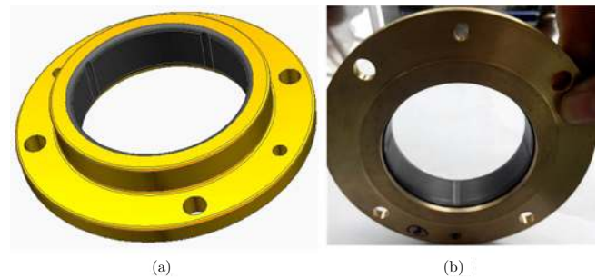
Fig. 10. Three dimensional model and physical map of test bearing.
