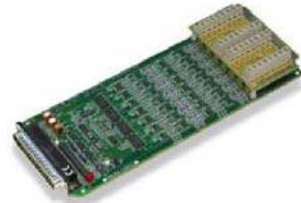
DBK82: 14-channel card with on-board screw terminals
