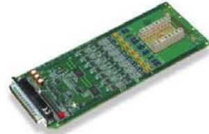
DBK81: 7-channel card with on-board screw terminals
