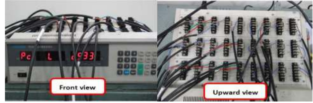
Fig. 5 static strain test instrument (YJ-22)
