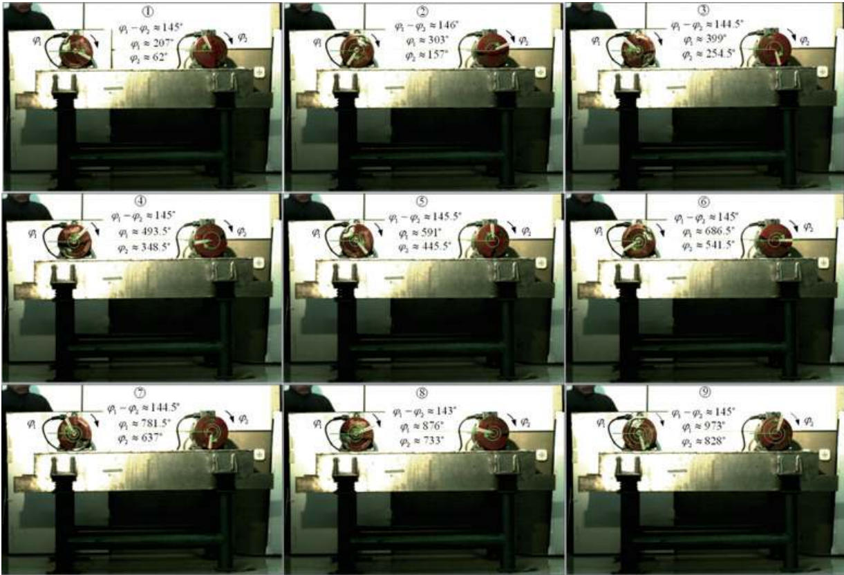
Fig. 9. The phases recorded by high-speed camera before the exciter 2 is cut off ( \eta = 0.5 ).
