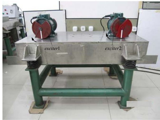
Fig. 7. A laboratory model of a vibrating system: (a) Schematic of experimental setup; (b) Vibrating synchronization bedstand.
