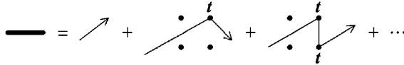
Fig. 6. Green's function G defined by the multiple scattering of a hole by impurities. G^{(0)} and t are the free propagator and t -matrix, respectively.
