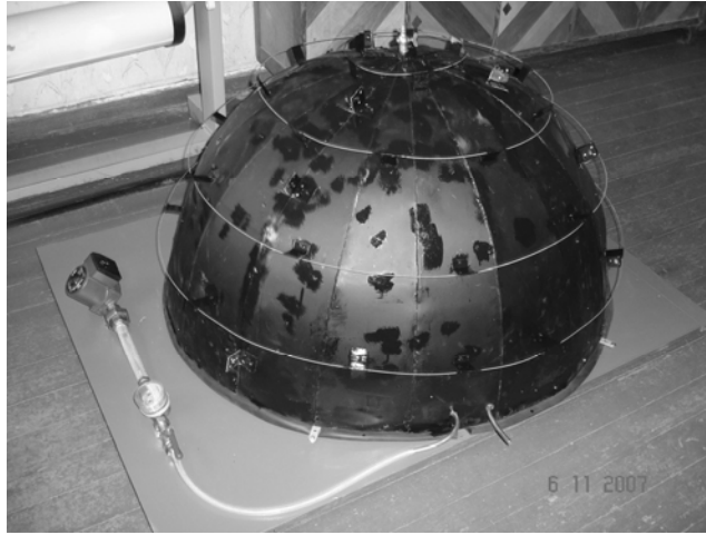
Fig. 2. Semi-spherical solar collector.
