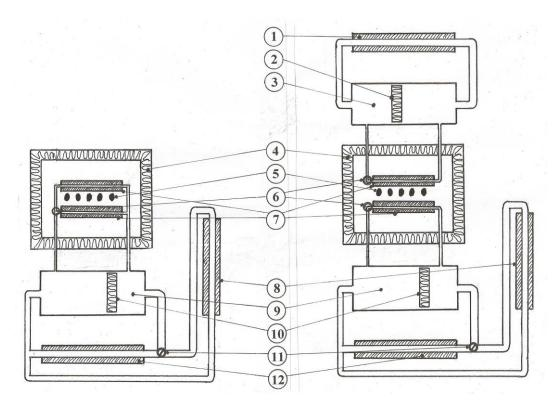
**Figure 1**. Schematic diagram of fair-trade sustainable mono-loop (left) and bi-loop (right) hatcheries. 1: nocturnal radiator, 2: cold separator, 3: cold water tank, 4: incubator, 5: eggs, 6: brooding regulator, 7: incubation exchanger, 8: heat discharge radiator, 9: hot water tank, 10: hot separator, 11: heat discharge regulator, 12: collector.
