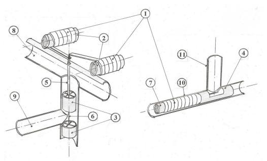
Figure 5. Incubation (left) and heat discharge (right) bimetallic-helix regulators.
