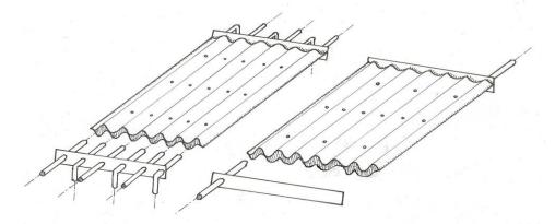
Figure 3. Corrugated sheet heat exchangers. Incubator exchanger with parallel circulation in alternating directions (left), collector and coil radiators (right).
