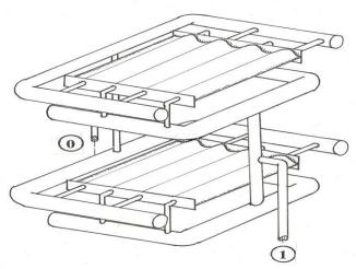
Figure 4. Incubator heat exchanger - Mono-loop version.
