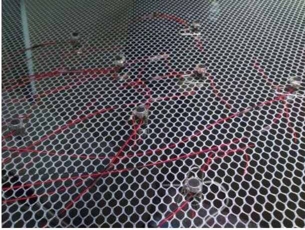
FIG. 7. (Color online) Implemented planar microphone array, using omnidirectional microphone pairs.
