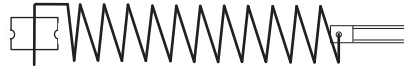
Figure D.4: Spring design: one end has a small teflon wheel attached, the other end a threaded rod for adjustability. The endpoint wires are twisted orthogonally to each other.
