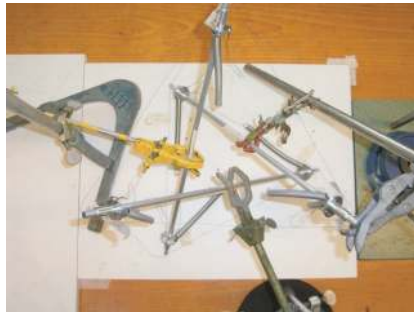
(a) When all springs are attached and all wirelengths are measured out, the bars are one by one firmly fixed with clamps ... (b) ... so that the springs can be tensioned
