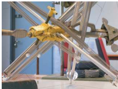
(c) Close-up of springs during assembly. (d) Removing the clamps that fix the bars.
