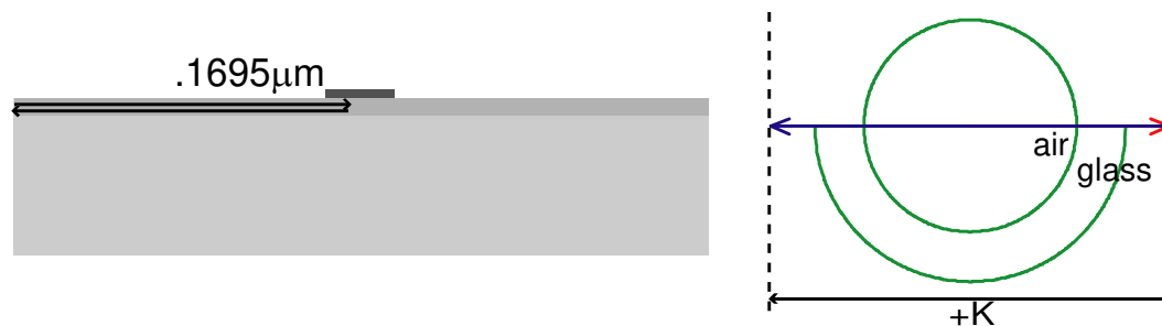
Figure 4.13 First order Bragg grating coupler
