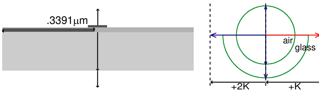
Figure 4.12 Second order Bragg grating coupler
