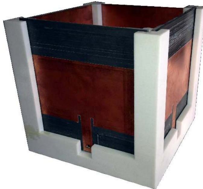
Figure 27: Photograph of the narrow-spacing microstrip patch array in 3D printed mount.
