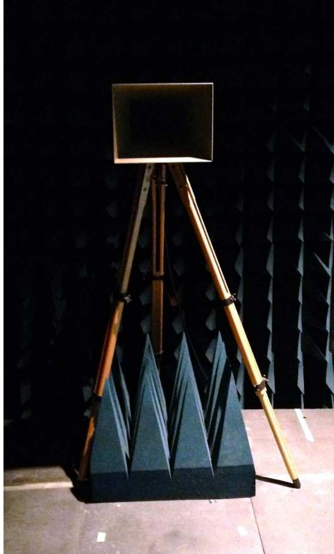
Figure 34: Standard gain horn antenna (ETS-Lindgren model 3160-03) used as the transmitter in the anechoic chamber. The flat surface upon which the antennas are mounted are walkway absorbers (i.e., RAM with a flat support structure on top).
