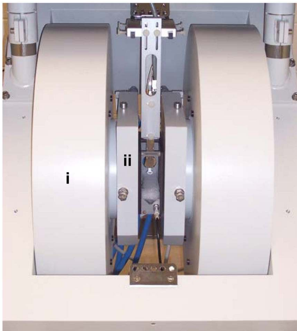
Figure 5. Bruker (Bruker BioSpin, Billerica, MA, USA) L-band EPR imager. Main magnet (i) and magnetic field gradient assembly (ii).
