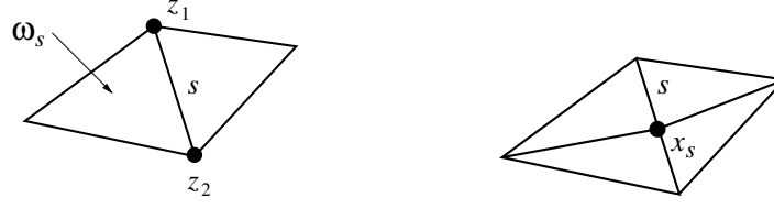
Fig. 12 Patch \omega_S of triangles associated to interior side (left) and its refinement for Dörfler cut-off function (right).
