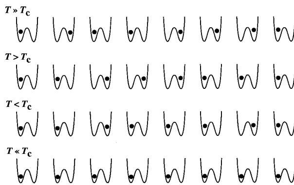
FIGURE 5. Sequence showing the ordering of atoms for the model of Figure 3 in the order-disorder limit. At high temperatures ( T \gg T_c , \eta = 0 ) the positions of neighboring atoms are not correlated in any significant way. On cooling toward the transition temperature ( T > T_c , \eta = 0 ) the effects of nearest-neighbor interactions become more significant and a degree of short-range order is established. Below the transition temperature ( T < T_c , |\eta| > 0 ) the probability is greater that one side of the double-well potential (in this case the left-hand side) will be occupied, but there is also a significant probability that some atoms will occupy the alternative potential well. At very low temperatures ( T \ll T_c ) most of the atoms occupy the same side of the double-well potential.
