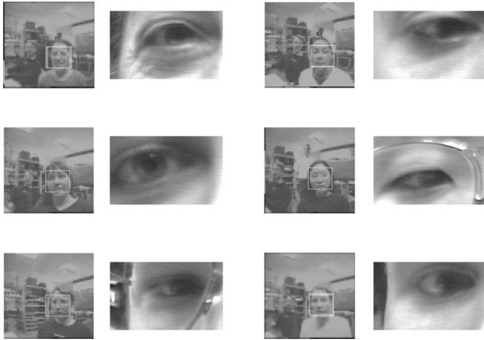
Figure 6. A selection of faces and eyes identified by the robot. Faces are located in the wide-angle peripheral image. The robot then saccades to the target to obtain a high-resolution image of the eye from the narrow field-of-view camera.
