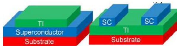
Fig. 8.1. Schematic of a TI grown epitaxially on a superconductor (left) and a superconductor film layered on a TI film [109].
