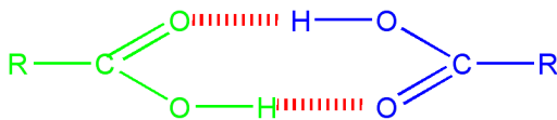
Fig. 4. Carboxyl group at surface of MWCNTs become hydrogen bond. The dotted line stands for hydrogen bond.
