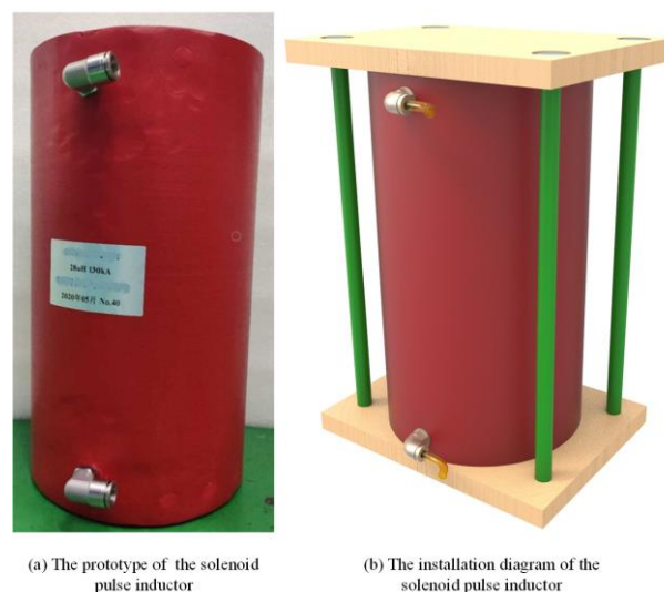
FIGURE 1. The prototype and installation diagram of the solenoid pulse inductor.
