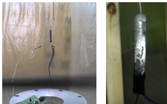
Fig. 3. General view of the test item before energization and after testing (charred).
