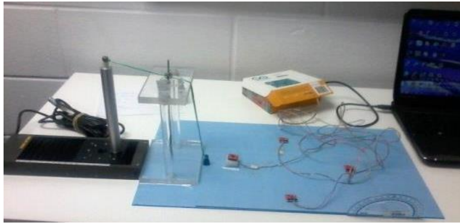
Figure 7-3 Experimental setup using four accelerometers for estimating tilt angles
