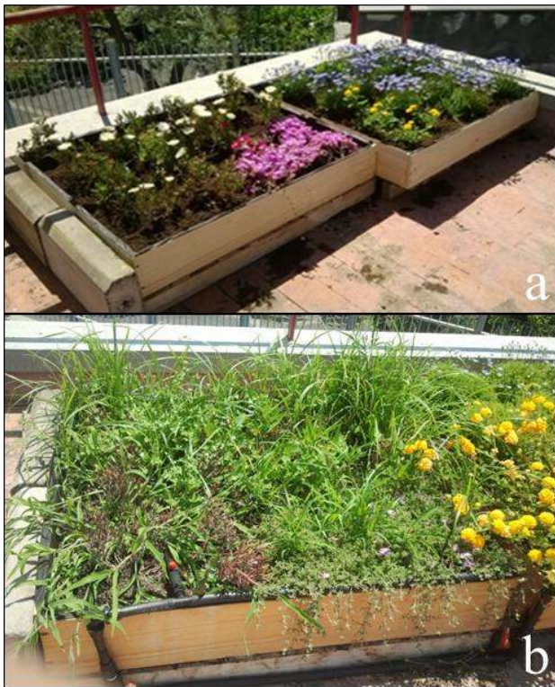
Figure 2. Prototype of green roof, a) Configuration at the installation time, b) Situation during the warmest week
