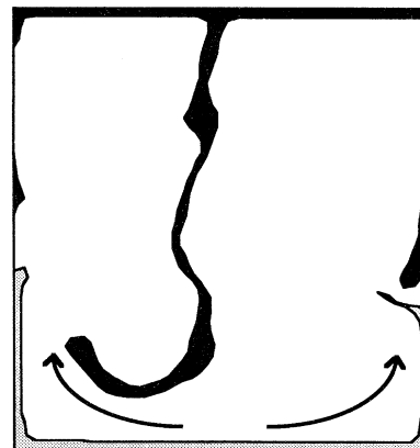
FIG. 6. Example of the dominant thermal features with single-vortex forcing. This sketch is based on liquid-crystal thermography. The secondary flow advects warm fluid (light shading) up along the side walls of the cell and creates a non-bursting lower boundary layer. Cool thermal plumes (dark shading) falling from the top are unopposed and frequently span the full height of the cell.
