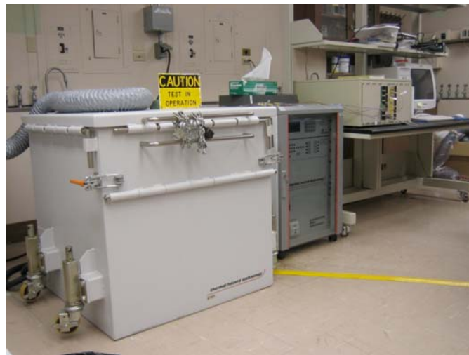
The blast enclosure and control rack of the ARC and the Arbin cycler
