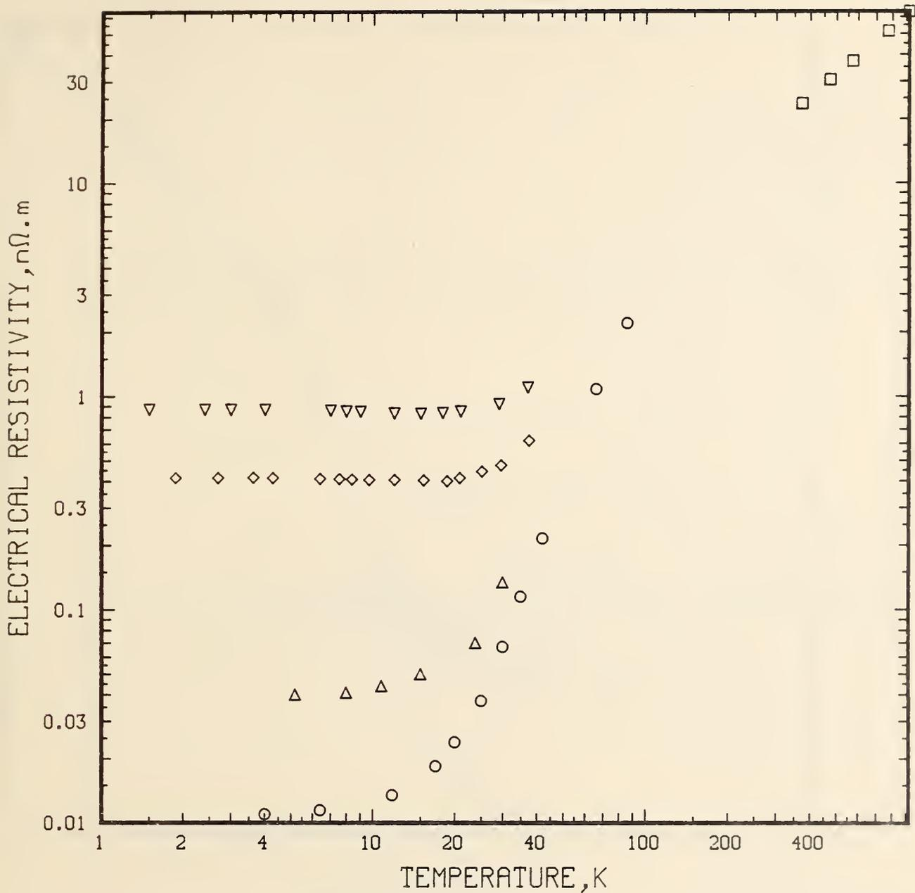
Figure 2.3.2 Experimental electrical resistivity data for copper selected from the following references in the copper annotated bibliography: (33,38,43)
