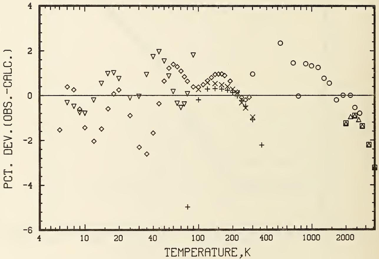
Figure 5.3.4 Electrical resistivity deviations of the tungsten data from the following references compared to eq. (1.2.3): (5A,11,14,22)
