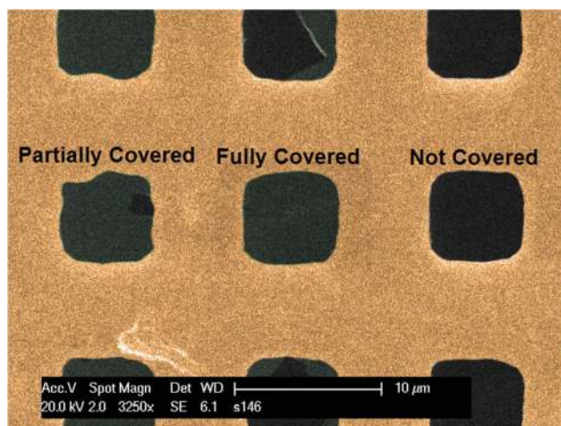
Fig. 1 Scanning electron microscopy image of graphene transferred on gold TEM grid showing 7.5 \mu\text{m} array of square holes. Some holes are fully or partially covered with the graphene flake. The grid is depicted in gold color, the holes are shown in black and the almost transparent greenish areas are suspended graphene flakes.
