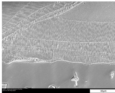
Figure 71. SEM image of the weld pool taken at 500X for the LSM specimen
