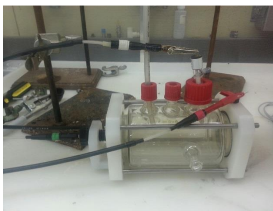
Figure 30. Installation of the corrosion cell system
