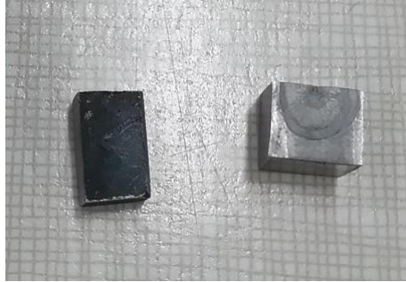
Figure 42. As received Solution annealed specimen (left). As received TIG melted specimen (right)
