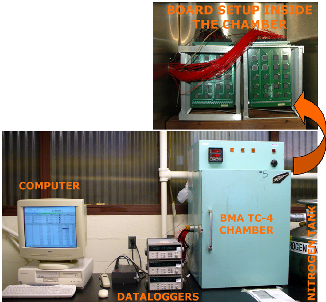
Figure 9. Thermal cycling test setup
