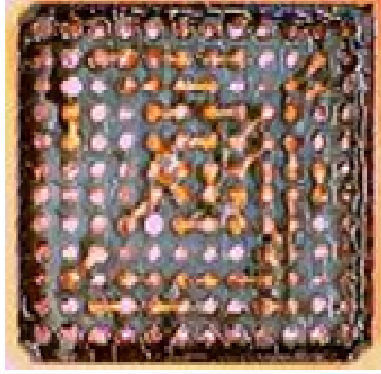
Figure 27. Optical picture of the pried 144 I/O BGA package in Sn based finished Sn3.5Ag soldered board (courtesy: CALCE)
