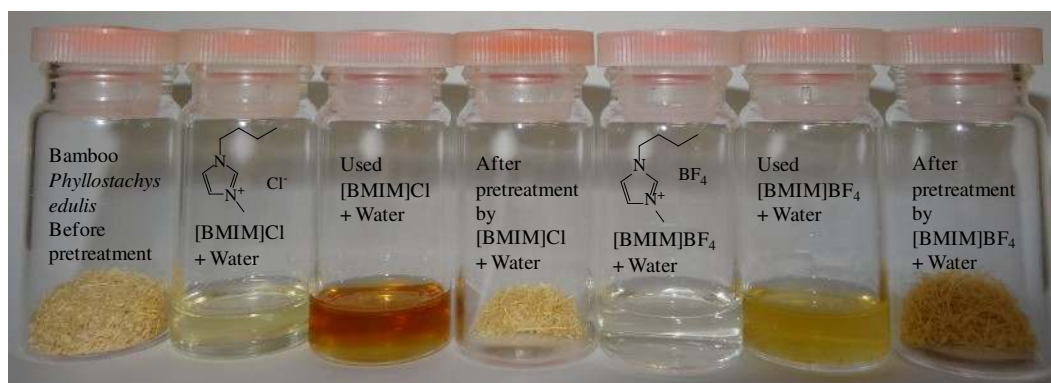
Figure 2. Appearance of bamboo samples before and after the pretreatment in [BMIM]Cl+water and [BMIM]BF 4 +water mixtures.
